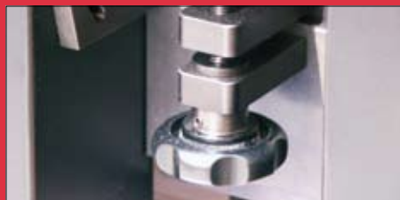
The disc wear is adjusted using a hand wheel with a threaded spindle. The facet angle can be adjusted using a motorised system.
