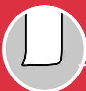
Sheet with burr after cutting
